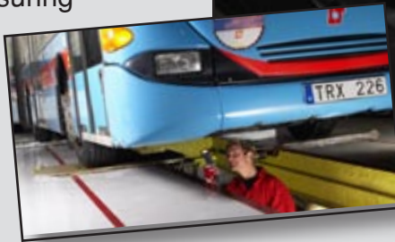
The play detector on the left is a useful accessory for checking that the bushings and bearings are free from excessive play before the wheel alignment.
