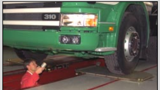
Before measuring wheel angles, the play detectors are used to check for worn parts.
